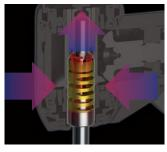
Unique, multi-point chuck MORITA's unique chuck design grips the bur firmly and doesn't lose its strength even after years of use. Experience the stability only a TORQTECH can provide when performing work that requires great precision.
